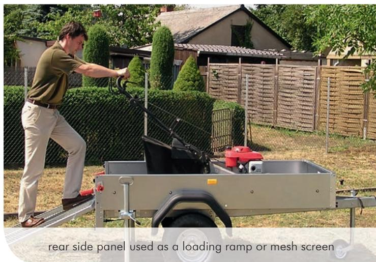
rear side panel used as a loading ramp or mesh screen
