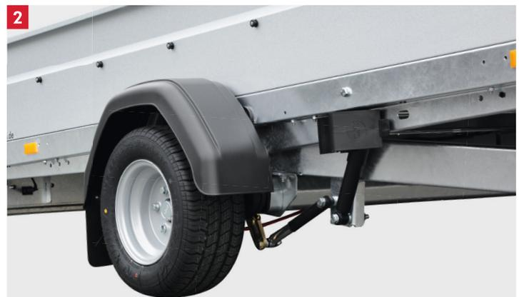
When travelling upwards and downwards with a vehicle the centre of gravity changes. As a result of this the tilting bridge raises or lowers.
