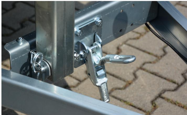
Attachment of the tipper bridge using safety release fastener.
