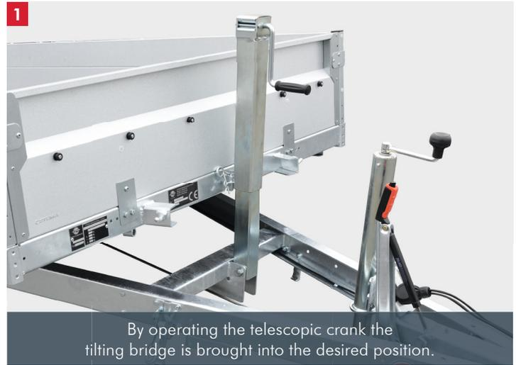
By operating the telescopic crank the tilting bridge is brought into the desired position.
