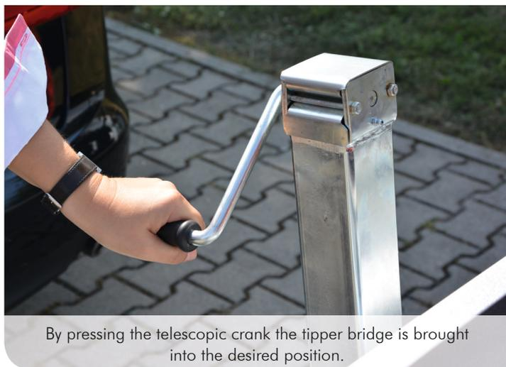
By pressing the telescopic crank the tipper bridge is brought into the desired position.
