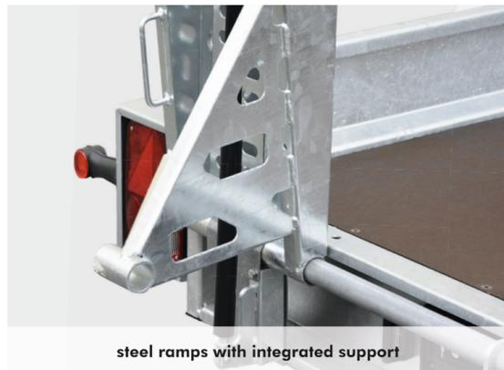
steel ramps with integrated support
