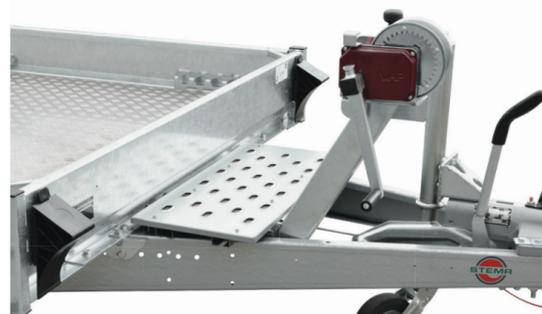
excavator bucket plate & winch stand with 12.5 m long cable (additional equipment)
