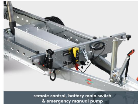
remote control, battery main switch & emergency manual pump
