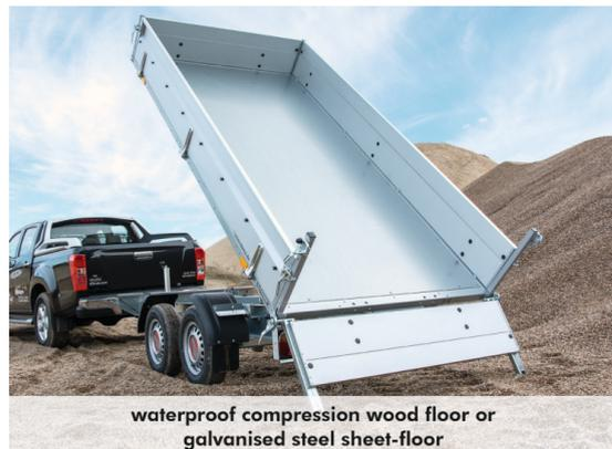
waterproof compression wood floor or galvanised steel sheet-floor
