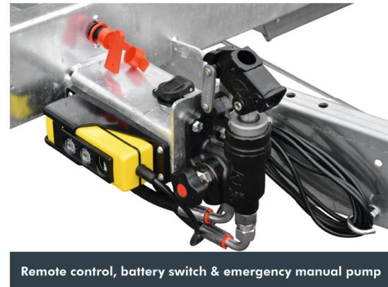
Remote control, battery switch & emergency manual pump
